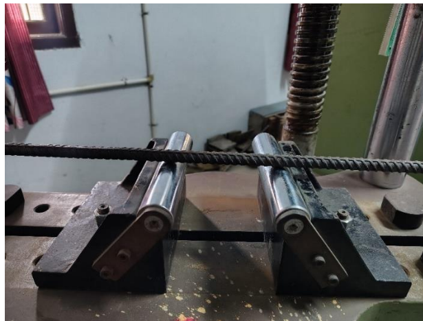
Figure 2: Bend Test Conducted on UTM
