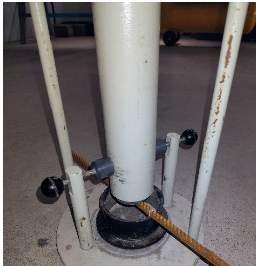
Figure 1: Drop Weight Impact Test
