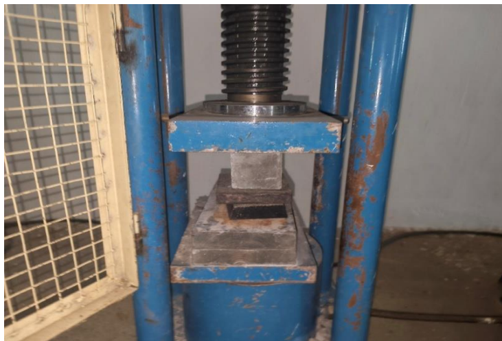
Figure 1: Compressive Testing Equipment
