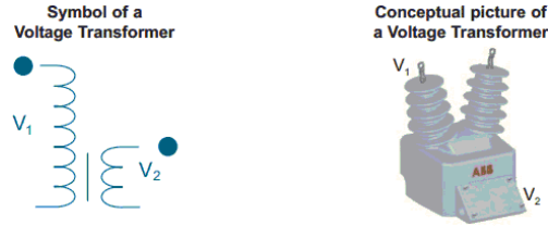
Fig. 3.1 Potential transformer or voltage transformer
