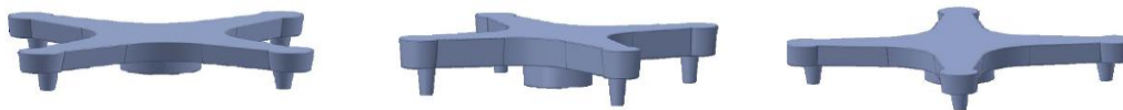
Figure 6: CAD Models Of 3 Sample Drone Positions In The Experimental Scenarios: Drone Faces The Laser Sensor (Top), The Drone Is Rotated By 22.5° (Middle) And 45° With The Sensor
